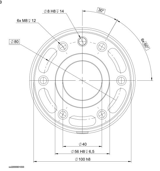
3.3.10 Fitting equipment on the robot (robot dimensions)
