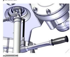
2 Hold the motor shaft still by inserting a pin through the joints (5-axis robot) or through the joint and against the casting. Choose an appropriate material for the pin, that
