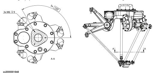
3.3.10 Fitting equipment on the robot (robot dimensions)
