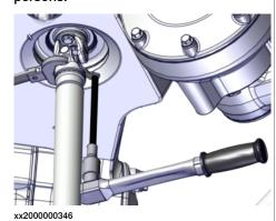
2 Hold the motor shaft still by inserting a pin through the joints (5-axis robot) or through the joint and against the casting. Choose an appropriate material for the pin, that does not damage the surface of the joints.
